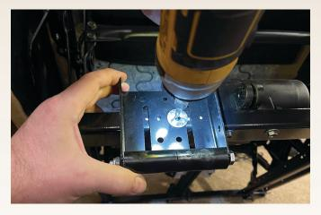
Final step is to attach the roller with self-tapping screws or bolt through the frame with nuts and bolts (not shown).
