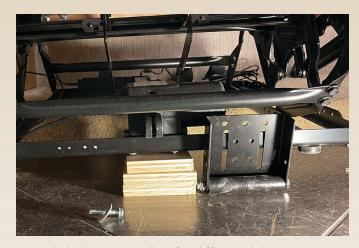
Multiple hole patterns allow for different slide heights 2"- 3.5"
