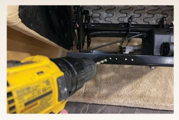
Optional drill can be used to drill smaller pilot holes for screws or holes for mounting with nuts and bolts.
