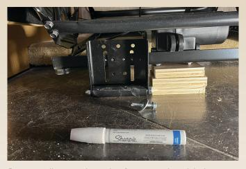
Position roller on either side of motor and mark holes. Can be mounted with either 2 or 4 screws or nuts and bolts.
