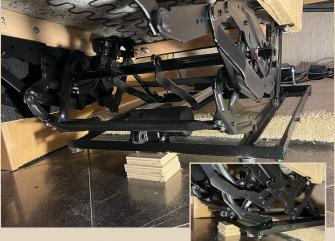
Use wood blocks or similar to level frame with the slideout.
