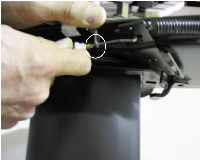
Step 4 Pull back on cable and insert it through slot on bottom of bracket
