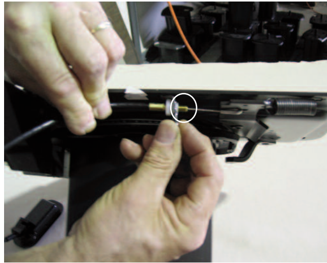
Step 5 Push clevis clip onto groove on nylon nut (on right side of bracket)
